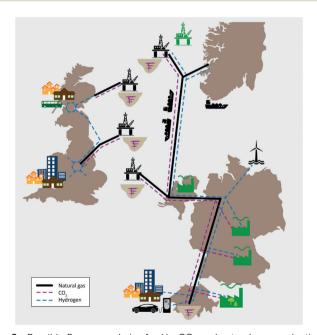
Fig. 2 Possible European chains for H<sub>2</sub>, CO<sub>2</sub> and natural gas production, transport, storage and usage. This map illustrates the large number of choices that must be made about the future energy system: where will  $H_2$ be produced, how will it be transported and used; how will CO2 be captured and transported, and where will it be stored?
