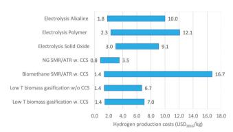
Fig. 3 Current reported cost ranges for selected hydrogen production technologies. Ranges based on values reported in Speirs et al., 131 IEA, 126 Binder et al., 132 Howes et al., 133 Bauer et al., 134 IEAGHG 135 and Parkinson et al. 136,137 and converted to 2016 USD per kg using an average 2016 USD/ GPB exchange rate of 1.3552 and an average 2016 EUR/GBP exchange rate of 1.1068.
