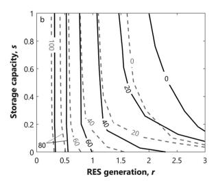
Fig. 1  $CO_2$  emissions isolines (in t per GWh<sub>el</sub>) at varying undispatchable renewable generation (*x*-axis) and storage capacity (*y*-axis) when considering a system with only H<sub>2</sub> storage (solid lines) and H<sub>2</sub> storage + batteries (dashed lines). Adapted from Gabrielli *et al.*<sup>64</sup>
