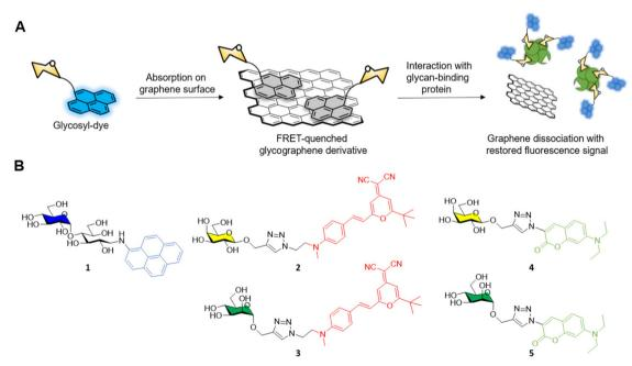
Fig. 1 (A) General principle for graphene and graphene derivatives-based FRET fluorescent glycoprobes used for glycan-binding protein sensing. (B) Structure of aminopyrene-1, dicyanomethylene-2 and 3, and aminocoumarin-4 and 5 glycoside derivatives.
