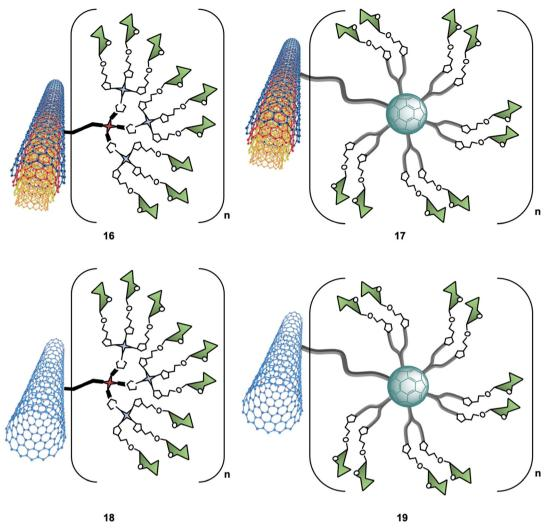
Structures of glyconanomaterials 16-19. For the sake of clarity, a nanotube fragment with one copy of glycodendron or glycofullerene is shown.
