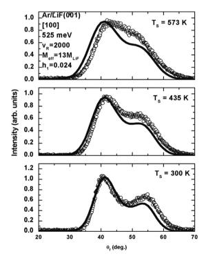
**Fig. 8** Angular distributions for Ar scattering from LiF(001) in the [100] direction at three different temperatures from 300 to 573 K as marked. The incident energy is 0.525 eV. There is a fixed angle of 90° between the incident beam and detector direction. The experimental data are shown as open circles and the solid curves are calculations using eqn (17) with a corrugation parameter h = 0.024. (Reprinted with permission from ref. 88, Copyright [2015] Elsevier.)
