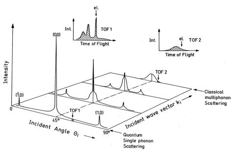
Fig. 1 A depiction of the transition from quantum mechanical scattering (in the front) to classical scattering (in the rear) as a function of increasing incident particle wave vector (increasing energy). At low incident energies, sharp quantum features are observed in both the angular distributions and the energy-resolved TOF1 and TOF2 plots (insets), while at large energy only broad classical features appear. Courtesy of J. R. Manson and J. P. Toennies.
