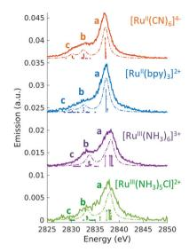
Fig. 6 Experimental (solid lines) and simulated (dashed lines) 4d → 2p VtC-XES spectra of a series of Ru(II) and Ru(III) complexes with low-spin d<sup>6</sup> and d<sup>5</sup> configurations, respectively. A global shift of 96.3 eV is applied to the calculated spectra. Reproduced with permission from ref. 102. Copyright 2021 Royal Society of Chemistry.
