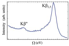
Fig. 4 A typical VtC X-ray emission spectrum showing  $K\beta''$  and  $K\beta_{2.5}$ features (experimental spectrum of [Cr<sup>III</sup>(NH<sub>3</sub>)<sub>6</sub>]<sup>3+</sup> adapted from ref. 118). The baseline of the spectrum is not horizontal because the exponential tail of the strong KB mainline has not been subtracted. Reproduced with permission from ref. 119. Copyright 2015 American Chemical Society.
