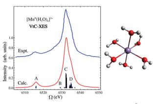
Fig. 5 Experimental and simulated VtC-XES spectra of [Mn<sup>II</sup>(H<sub>2</sub>O)<sub>6</sub>]<sup>2+</sup>. Simulated results have been red-shifted by 30.4 eV to match experiment. 120 The molecular structure is shown on the right. Color code: O (red), Mn (purple), H (white). Reproduced with permission from ref. 119. Copyright 2015 American Chemical Society.
