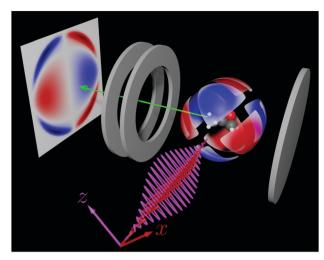
Fig. 4 Proposed velocity map imaging setup to measure the coefficient  $ilde{b}_{3,-2}$ :  $\omega$  (red wave) and  $2\omega$  (violet wave) are polarized along x and z, respectively. The detector projects the distribution on the x = z plane. Only the contribution of  $\tilde{b}_{3,-2}$  to the photoelectron angular distribution is shown. In red/blue regions there is an excess/deficit of photoelectrons.
