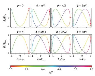
Fig. 2 Lissajous curves of the field (2) for different values of  $\phi$ . The position of the red arrow indicates t=0.
