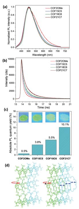
Fig. 2 (a) Solid state photoluminescence spectra, (b) fluorescence decay curves, (c) absolute fluorescence quantum yield with inset fluorescence images of COF2OMe, COF15C5, COF18C6 and COF21C7 powders. (d) Schematic presentation of backbone rotation restriction by stacking of semi-rigid crown ether chains (red arrow indicates possible rotation mode, blue arrows represent repulsion force).
