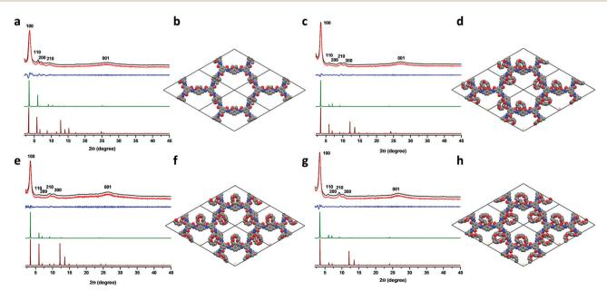
Fig. 1 Powder XRD patterns of experimental (black), Pawley-refined (red), their difference (blue), simulated eclipsed (green) and staggered (brown) stacking for (a) COF2OMe, (c) COF15C5, (e) COF18C6 and (g) COF21C7. Simulated crystal structures of (b) COF2OMe, (d) COF15C5, (f) COF18C6 and (h) COF21C7.
