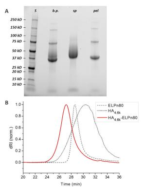
**Fig. 2** Characterization of the  $HA_{4.6k}$ -ELPn80 bioconjugate by SDS-PAGE (A) and SEC (B). A: S: protein size markers; b.p.: reaction medium before purification; sp: supernatant; pel: pellet. B: samples in phosphate buffer.
