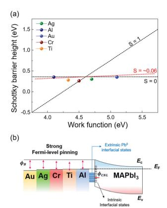
Fig. 5 (a) Extracted Schottky barrier heights of MAPbl<sub>3</sub> for the various metal work functions, showing the pinning factor  $S \sim 0.06$  when the deposited metal thickness is 40 Å (red dashed line). (b) Band diagram of metal/MAPbl<sub>3</sub> interfaces with five different metals.
