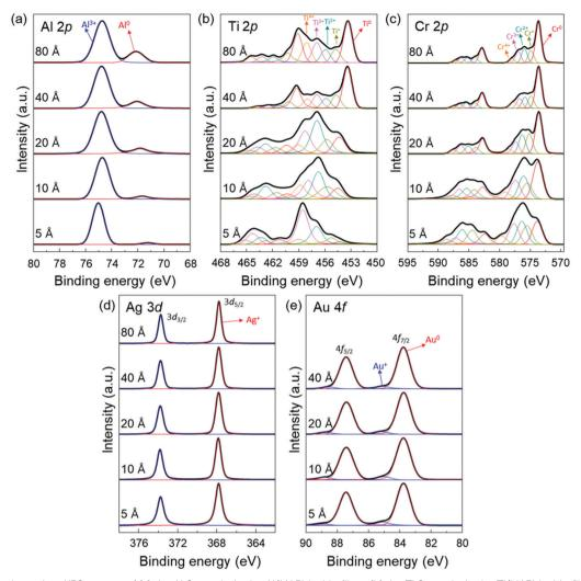
Fig. 3 Thickness dependent XPS spectra of (a) the Al 2p peaks in the Al/MAPbl<sub>3</sub> thin films, (b) the Ti 2p peaks in the Ti/MAPbl<sub>3</sub> thin films, (c) the Cr 2p peaks in the Cr/MAPbI<sub>3</sub> thin films, (d) the Ag 3d peaks in the Ag/MAPbI<sub>3</sub> thin films, and (e) the Au 4f peaks in the Au/MAPbI<sub>3</sub> thin films
