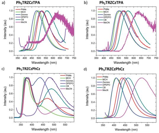
Fig. 3 Emission spectra of the compounds (a) Ph3TRZCzTPA, (b) Ph2TRZCzTPA, (c) Ph2TRZCzPhCz and (d) Ph3TRZCzPhCz in film and different solvents, methylcyclohexane (MCH), chlorobenzene (CB) and acetonitryl (MeCN).
