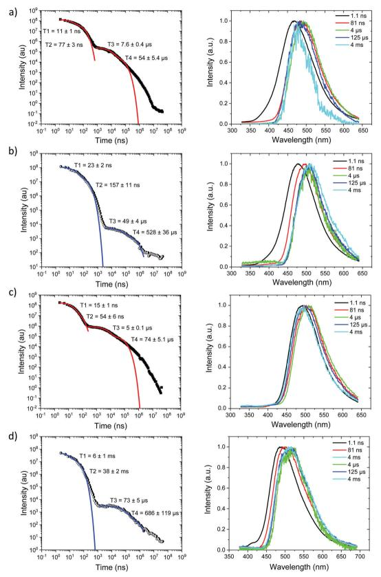
Fig. 4 Time-resolved spectrally integrated intensity decay (left) and representative time resolved spectra (right) of Ph<sub>3</sub>TRZCzTPA (a) 300 K and (b) 80 K; Ph2TRZCzTPA (c) 300 K and, (d) 80 K in zeonex matrix. Spectral times given in ns, and decay fitting data included in the decay plots.
