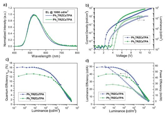
Fig. 9 (a) Normalized EL spectra at a luminance of  $10^3$  cd m<sup>-2</sup>; (b) current density-luminance-voltage (J-V-L) characteristics; (c) external quantum efficiency versus luminance, (d) luminance/power efficiency versus luminance for devices A and B.
