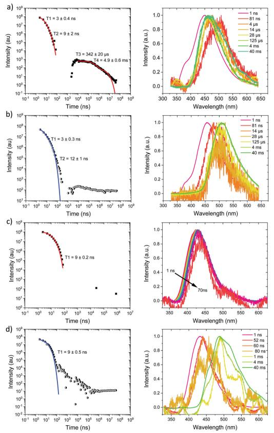
Fig. 5 Time-resolved spectrally integrated intensity decay (left) and representative time resolved spectra (right) of (a) Ph2TRZCzPhCz, (a) 300 K and (b) 80 K; Ph<sub>3</sub>TRZCzPhCz, (c) 300 K and, (d) 80 K in zeonex matrix. Spectral times given in ns, and decay fitting data included in the decay plots.
