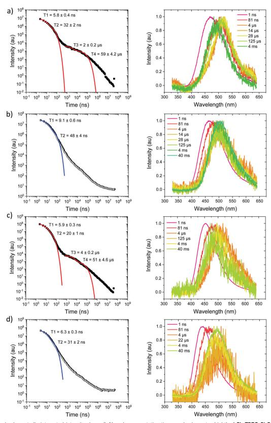
Fig. 7 Time-resolved spectrally integrated intensity decay (left) and representative time resolved spectra (right) of Ph2TRZCzPhCz, (a) 300 K and (b) 80 K; Ph<sub>3</sub>TRZCzPhCz, (c) 300 K and (d) 80 K in DPEPO host. Spectral times given in ns, and decay fitting data included in the decay plots.
