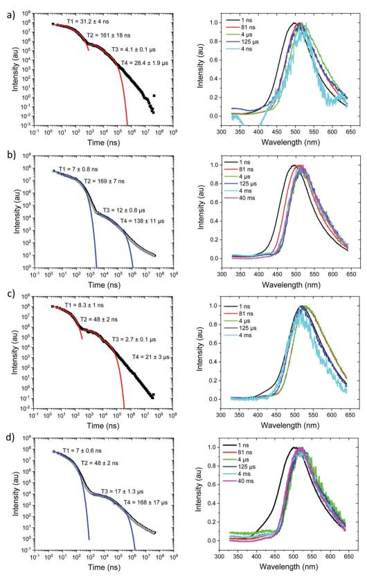
Fig. 6 Time-resolved spectrally integrated intensity decay (left) and representative time resolved spectra (right) of Ph<sub>3</sub>TRZCzTPA (a) 300 K and (b) 80 K; Ph2TRZCzTPA (c) 300 K and (d) 80 K in DPEPO host. Spectral times given in ns, and decay fitting data included in the decay plots.
