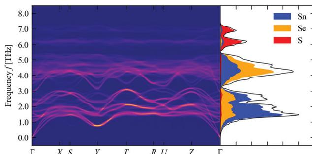
**Fig. 6** Unfolded dispersion and atom-projected density of states (PDOS) of  $\text{Sn}(\text{S}_{0.1875}\text{Se}_{0.8125})$ . The colour scale in the unfolded dispersion represents the spectral weight and runs from blue (low weight) to yellow (high weight).
