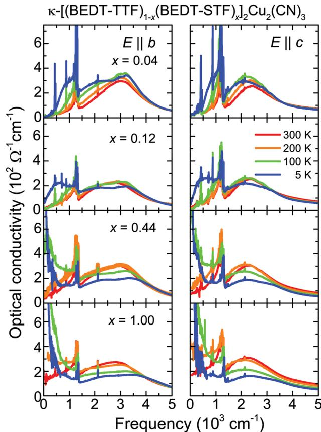
Fig. 4 Frequency dependent conductivity of  $\kappa$ -[(BEDT-TTF) $_{1-x}$ (BEDT-STF) $_x$ ] $_2$ Cu $_2$ (CN) $_3$  for several substitution values  $x = 0.04, 0.12, 0.44$ , and  $x = 1$  recorded for the two polarizations within the plane (left column  $E \parallel b$ ; right column  $E \parallel c$ ) at different temperatures as indicated in the legend.
