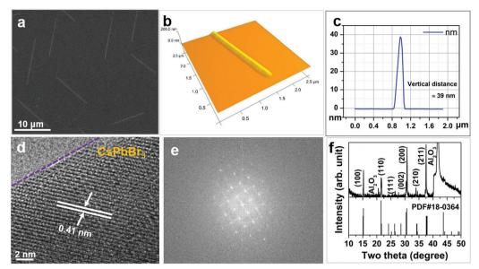
Fig. 1 (a) A field emission scanning electron microscopy (FESEM) image of CsPbBr<sub>3</sub> NWs grown on c-Al<sub>2</sub>O<sub>3</sub>. (b and c) An atomic force microscopy (AFM) image showing triangular morphology and the corresponding line scan showing the height of the nanowire. (d and e) A HRTEM image and the corresponding FFT pattern of a CsPbBr<sub>3</sub> NW. (f) An X-ray diffraction pattern from CsPbBr<sub>3</sub> NWs grown on c-Al<sub>2</sub>O<sub>3</sub>.
