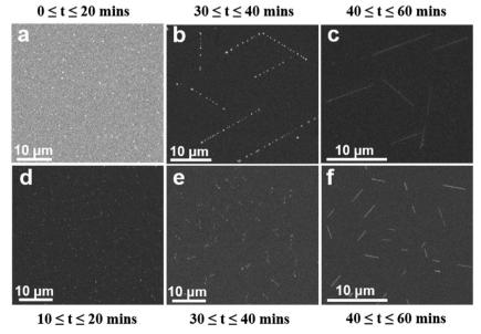
Fig. 3 Time evolution of CsPbX<sub>3</sub> (X = Br, Cl) perovskite nanowires in NC-CVD growth. (a-c) and (d-f) are the FESEM images of 3 different stages of the time evolution growth of CsPbBr<sub>3</sub> and CsPbCl<sub>3</sub> perovskite nanowires, respectively.
