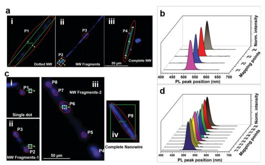
Fig. 6 Photoluminescence (PL) mapping and the corresponding PL spectra of CsPbBr<sub>3</sub> dot like spherical halide particles, incomplete NWs/NW fragments, and complete NWs grown respectively on (a and b) SiO<sub>2</sub>/Si- and (c and d) c-Al<sub>2</sub>O<sub>3</sub> substrate. P1 to P9 denote the PL measurement spots on different structures and/or position on the same structures. Color in the PL scanning map does not represent the real emission color.
