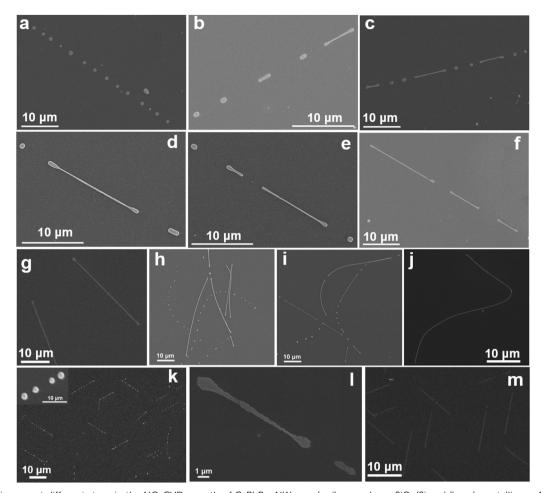
Fig. 2 FESEM images at different steps in the NC-CVD growth of CsPbBr<sub>3</sub> NWs on: (a-j) amorphous SiO<sub>2</sub>/Si and (k-m) crystalline c-Al<sub>2</sub>O<sub>3</sub> substrates. (g and j) and (m) show different final shapes of CsPbBr<sub>3</sub> NWs on SiO<sub>2</sub>/Si and Al<sub>2</sub>O<sub>3</sub> substrates, respectively.
