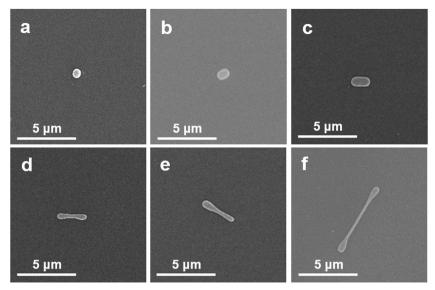
Fig. 5 (a-f) Successive transformations of CsPbBr<sub>3</sub> single halide particle into a stable dumbbell shape during the growth of single-crystalline halide nanowires by the NC-CVD
