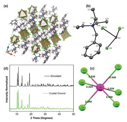
Fig. 3 XRD characterization of the (BzTEA)<sub>2</sub>TeCl<sub>6</sub> hybrid. Overview of the single crystal structure (a); asymmetric unit (b); site symmetry of Metal-Halide octahedron (c); comparison of the simulated and experimental PXRD pattern using Cu source (d). H atoms are omitted in (b) for clarity,
