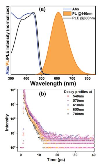
Fig. 2 Optical characterization of (BzTEA)<sub>2</sub>TeCl<sub>6</sub> showing (a) absorbance (Abs), photoluminescence (PL), and photoluminescence excitation (PLE) spectra; (b) lifetime decay profiles collected across the PL band ( $\lambda_{exc}$  = 440 nm).
