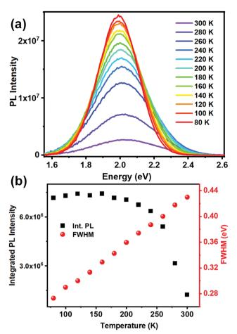
Fig. 4 (a) Low temperature PL ( $\lambda_{\rm exc}$  = 440 nm) spectra of (BzTEA)<sub>2</sub>TeCl<sub>6</sub> crystals; (b) integrated PL intensity and bandwidth (FWHM) as a function of temperature.
