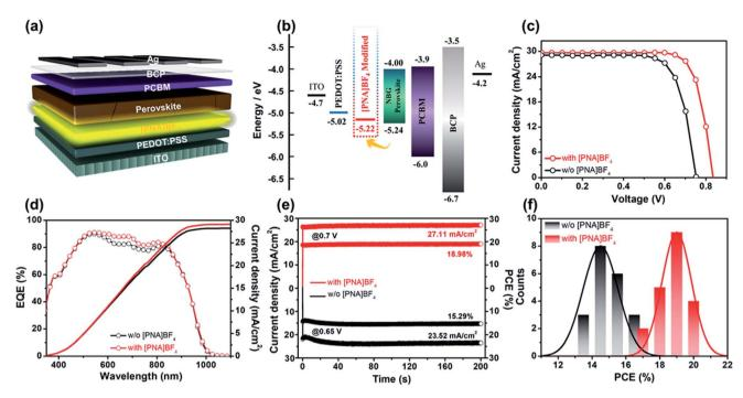
Fig. 4 (a) The device structure of mixed Sn-Pb perovskite PSCs treated by [PNA]BF4 ionic salts; (b) energy-level diagram of each layer related devices; (c) J-V curves of champion PSCs under AM 1.5G 100 mW cm<sup>-2</sup> illumination; (d) EQE spectra of corresponding PSCs; (e) steady-state  $J_{sc}$ and corresponding efficiencies of champion devices (at 0.70 V for the PSC with [PNA]BF4, at 0.65 V for the PSC without [PNA]BF4); (f) performance distribution diagram for 20 devices in one bath.
