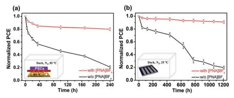
Fig. 6 (a) Thermal and (b) shelf stability of PSCs devices with or without [PNA]BF4 treatment.
