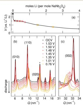
Fig. 7 (a) Galvanostatic discharge of NaNb<sub>3</sub>O<sub>8</sub> during operando X-ray scattering and (b and c) operando XRD at select states of charge, marked in (a), shows the evolution of specific reflections during lithiation (\* marks a reflection from a component of the operando cell). The y-axis in (b) and (c) corresponds to the intensity of X-ray scattering, which is shown here on a arbitrary scale.
