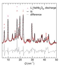
Fig. 10 Ex situ XRD of the first discharge product of NaNb<sub>3</sub>O<sub>8</sub> and a fit of the data based on a model with a decreased interlayer spacing and expanded c lattice parameter. The y-axis corresponds to the intensity of X-ray scattering, which is shown here on a arbitrary scale.
