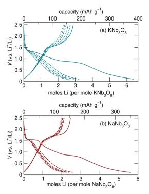
Fig. 6 Galvanostatic cycling of (a)  $KNb_3O_8$  and (b)  $NaNb_3O_8$ , with the first cycle in solid lines and increasingly broken lines for subsequent cycles. In their first cycle,  $KNb_3O_8$  and  $NaNb_3O_8$  have similar cycling profiles, consisting of a combination of plateaued and sloped regions, with asymmetry in the profiles between discharge and charge. Later cycling shows a slow fade in capacity for both compounds.
