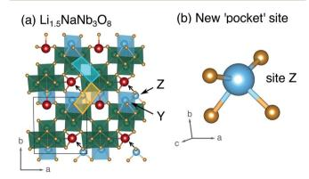
Fig. 12 (a) Structure of  $\rm Li_{1.5}NaNb_3O_8$  with Z sites filled, causing Li–Na repulsion and displacement of Na (red). (b) Geometry of the four-fold-coordinate Li ion in pocket site Z.
