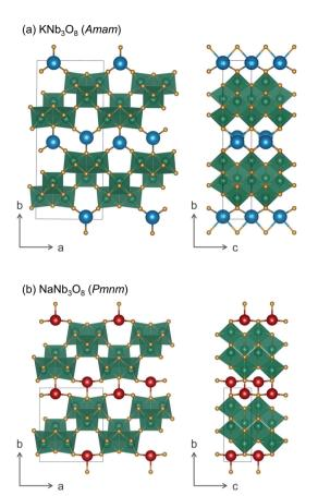
Fig. 2 In (a) KNb $_3$ O $_8$  and (b) NaNb $_3$ O $_8$ , Nb $_3$ O $_8$  layers are separated by counter-cations. The size and preferred coordination of counter-cation (K or Na) determine the interlayer spacing as well as the stacking sequence of adjacent layers, AB for KNb $_3$ O $_8$  (with B shifted by  $\frac{c}{2}$ ) and AA in NaNb $_3$ O $_8$ .
