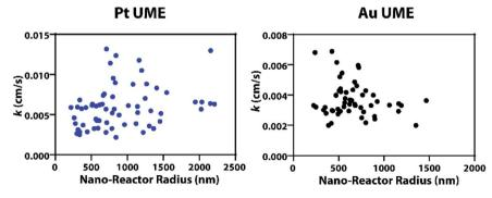
Fig. 2 Plots demonstrating the effect that aqueous nanodroplet size, filled with 50 mM CuCl<sub>2</sub> and glycerol (50%, v/v), has on the heterogeneous rate kinetics on a Pt and Au microelectrode. The large spread in the data without an observed trend indicates they are independent of nanodroplet size.
