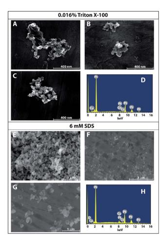
Fig. 3 SEM images and representative EDX spectra showing the morphologies of copper nanoparticles (NPs) deposited on platinum foil from aqueous nanodroplets containing 50 mM CuCl<sub>2</sub> with added surfactants in a continuous phase of 0.1 M [TBA][PF $_6$ ] in 1,2-DCE. (A–D) SEM data and corresponding EDX using an added surfactant of 0.016% w/v Triton X-100. (E–H) SEM data using an added surfactant of 6 mM SDS (r=28 nm  $\pm$  11 nm).
