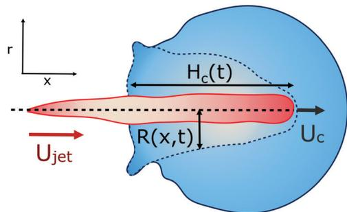
Fig. 4 Diagram illustrating the parameters used in this section. The jet impacts the pendant droplet from the left with velocity  $U_{\text{jet}}$ , creating a cavity with increasing depth in time  $H_c(t)$ , where the velocity of the apex of the cavity is indicated by  $U_c = \dot{H}_c$  and whose radius depends on time and the position  $R(x, t)$ . Here,  $x$  is the direction along which the jet travels and  $r$  is its perpendicular radial direction.
