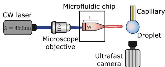
**Fig. 2** Schematic of the experimental setup. Thermocavitation is obtained focusing a CW laser on the bottom of a microfluidic device with a microscope objective. The thermocavitated bubble expands and creates a liquid jet that is directed at a pendant droplet. The process is recorded with a high-speed camera with the illumination coming from a light source from the front so the cavity evolution can be observed.
