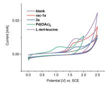
Fig. 4 Cyclic voltammogram of several reactants in AcOH with  $n Bu_4 NPF_6$  (0.1 M) at 100 mV s  $^{-1}$ .
