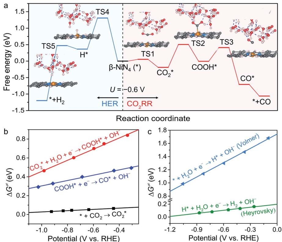
Fig. 4 (a) Free energy diagram of the  $\text{CO}_2\text{RR}$  and competing HER on  $\beta\text{-NiN}_4$  at  $U = -0.60$  V. The insets are snapshots of the transition states (TS). The arrow symbols indicate the directions of the HER and  $\text{CO}_2\text{RR}$  processes. (b and c) Calculated kinetic barriers  $\Delta G^\ddagger$  for the (b)  $\text{CO}_2\text{RR}$  and (c) HER on  $\beta\text{-NiN}_4$  as a function of the electrode potential  $U$ .
