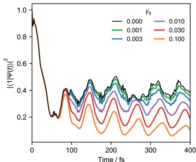
Fig. 6 Electronic populations of pyrazine, using the LVC Hamiltonian and different system-bath couplings  $\gamma_0$ , all at a temperature of 300 K. As  $\gamma_0$  is increased, the details of the closed-system result ( $\gamma_0 = 0$ ) are lost and the coherent oscillations are damped.
