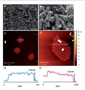
Fig. 3 (a) and (b) SEM images of bulk 1 and  $2 \cdot TP$  respectively. Scale bars represent 10  $\mu$ m. (c) and (d) selected AFM topographical images of the nanosheets formed from exfoliation of 1 and  $2 \cdot TP$  respectively. (e) and (f) height profiles of the nanosheets shown in (c) and (d) (represented by white bars).
