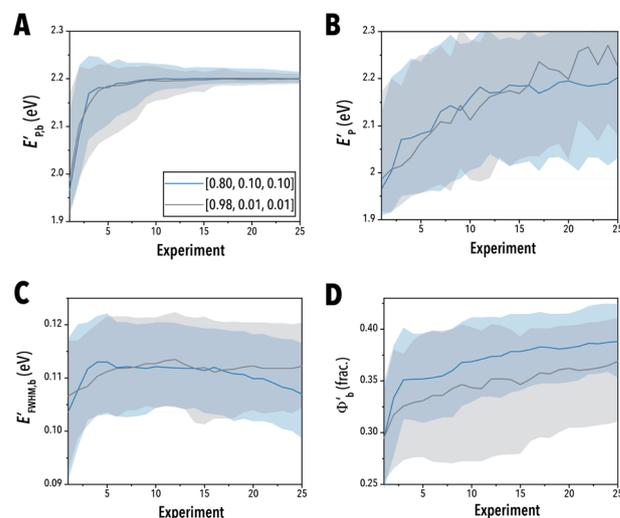
Fig. 6 (A) Median of the best observed peak emission energy, (B) the peak emission energy, (C) best observed emission full-width at half-maximum, and (D) best observed photoluminescence quantum yield as determined by the data weights [0.8, 0.1, 0.1] for a both balanced and peak emission biased utility function sampling with EI. The shaded regions correspond to the 25<sup>th</sup> and 75<sup>th</sup> percentiles of the simulated replicates.
