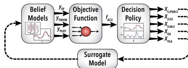
**Fig. 4** Illustration of the AI-guided material synthesis algorithm applied in this work. Experimental data from the surrogate model are used to train the belief model (either an ensemble neural network or Gaussian process regression) on the three output parameters, which are converted into a single quality value through the objective function. The response of this model is evaluated through the decision policy, which is used to select the next set of experimental conditions.
