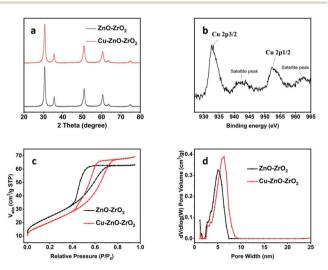
Fig. 1 PXRD patterns (a), high-resolution XPS of Cu element (b), nitrogen isotherms (c), and pore size distribution (d) for the catalyst Cu–ZnO–ZrO<sub>2</sub> and the pristine bimetal oxide support ZnO–ZrO<sub>2</sub>.
