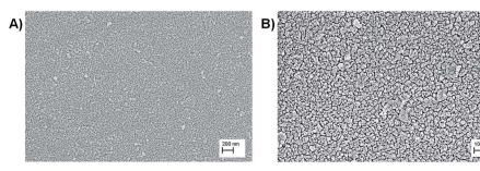
Fig. 2 SEM imagines of PEDOT-C<sub>60</sub> polymer film at different magnifications: (a)  $23\,000\times$ , and (b)  $57\,000\times$ .
