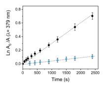
Fig. 5 First-order kinetic data fitting for the photooxidation of DMA in DMF sensitized by PEDOT- $C_{60}$  ( $\blacksquare$ ) and fullerene  $C_{60}$  ( $\blacksquare$ ).  $\lambda_{irr}=455-800$  nm. Values represent mean  $\pm$  standard deviation (error bars) of three consecutive experiments.
