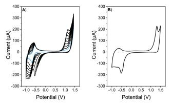
Fig. 1 (A) Repetitive cyclic voltammograms of a 0.5 mM solution of EDOT- $C_{60}$  in TBAPF<sub>6</sub> (0.1 M)/DCM. Light blue line denotes the first cyclic voltammogram. (B) Cyclic voltammogram of a PEDOT- $C_{60}$  film electro-deposited on ITO electrode in TBAPF<sub>6</sub> (0.1 M)/DCM. Scan rate: 50 mV s<sup>-1</sup>.
