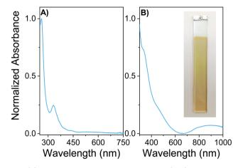
Fig. 3 (A) Electronic absorption spectrum of EDOT-C<sub>60</sub> monomer in DCM at room temperature. (B) Absorption spectrum of PEDOT-C<sub>60</sub> film on ITO. The inset shows a photo of the polymer PEDOT-C<sub>60</sub> deposited on ITO
