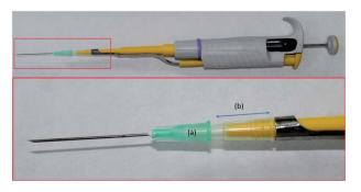
Fig. 1 Image of the attachment of the PDA-coated hypodermic needle to the micropipette. The Luer connector of the hypodermic needle (a) is connected to the micropipette using a section of a 100  $\mu$ L plastic tip (b). This device is used for needle conditioning and elution when a lower volume of solutions is required. For sample processing, however, the needle is attached to a 2 mL disposable plastic syringe.
