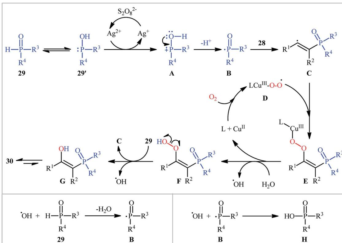
Scheme 13 Mechanistic proposal from the formation of  $\beta$ -ketophosphoryl compounds **30**.
