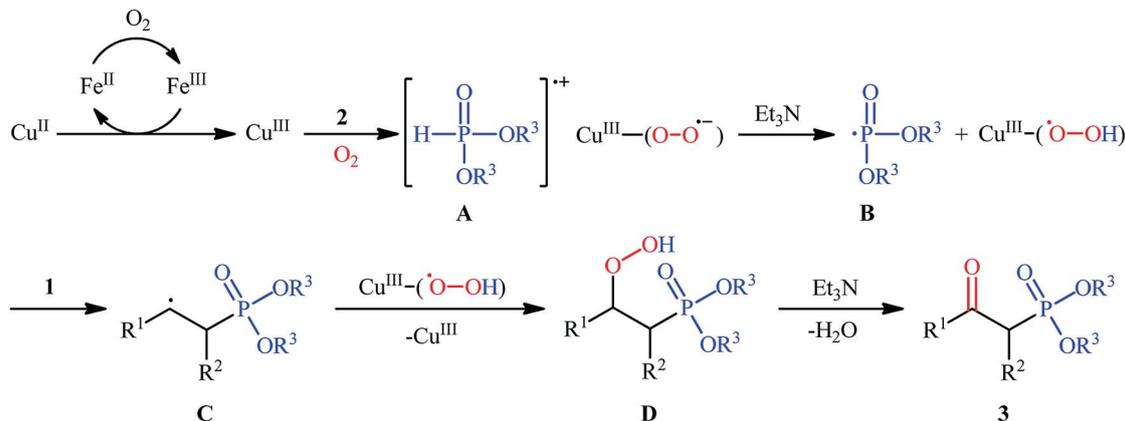
Scheme 3 Possible mechanism of Cu-catalyzed oxyphosphorylation of alkenes **1** with H-phosphonates **2** and O<sub>2</sub>.
