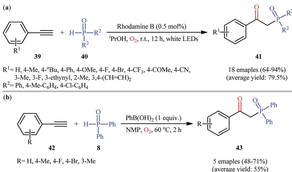
Scheme 16 (a) Visible-light-mediated oxidative coupling of terminal alkynes **39** and diaryl phosphine oxides **40**; (b) PhB(OH)<sub>2</sub>-mediated oxyphosphorylation of aromatic terminal alkynes **42** with diphenylphosphine oxide **8**.
