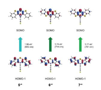
Fig. 11 TDDFT calculated molecular orbital transitions of most bathochromic absorptions of radical cations  $5^{++}$ ,  $6^{++}$ , and  $7^{++}$  (uB3LYP/6-311++ $G^{**}$ , IEFPCM CH<sub>2</sub>Cl<sub>2</sub>, isosurface value 0.05 a.u.) (For further molecular orbital transitions, see SI).
