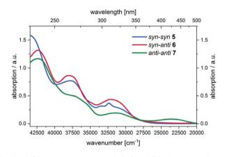
Fig. 5 UV/Vis spectra of compounds 5, 6, and 7 in the spectroelectrochemical cell at zero potential ( $CH_2Cl_2$ , T = 293 K).
