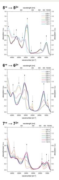
Fig. 8 UV/Vis spectroelectrochemical measurements of radical cations  $5^{++}$ ,  $6^{++}$ , and  $7^{++}$  forming the corresponding dications  $5^{2+}$ ,  $6^{2+}$ , and  $7^{2+}$  $(CH_2Cl_2, T = 293 \text{ K}; \text{ electrolyte } 0.1 \text{ M} [^nBu_4N][PF_6]; \text{ Pt working electrode,}$ Pt counter electrode and Ag/AgCl pseudo reference electrode).
