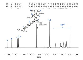
Fig. 3 <sup>1</sup>H NMR spectrum (700 MHz, CD<sub>2</sub>Cl<sub>2</sub>) of cage (R,R)-9. # residual CH2Cl2.
