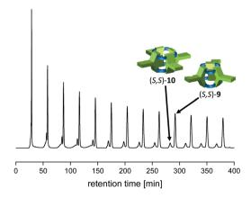
Fig. 2 Recycling-GPC chromatogram of the reaction of 7 with (S,S)-8. For experimental details, see ESI.† Please note that in between the peak at 150 min and 160 min, the compounds responsible for the broad peak were removed.
