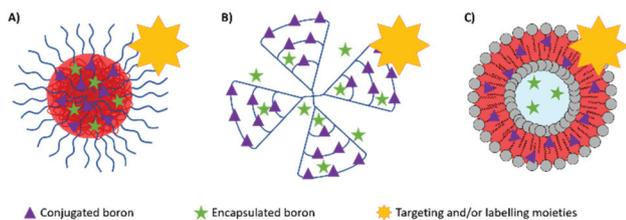
**Fig. 3** Overview of the various polymeric systems containing boron, either conjugated or encapsulated, and the possible conjugation to targeting or labelling moieties: (A) micelles made from polymers or dendronised polymers; (B) dendrimers; and (C) liposomes.
