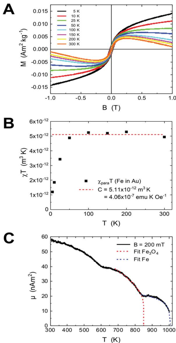
**Fig. 5** Magnetic characterization of AuFe NPs. (A) Hysteresis loops recorded at various temperatures between 5 K and 300 K. (B)  $\chi T(T)$  plot after subtraction of the Au diamagnetic component for the evaluation of the Curie constant; (C) high-temperature total magnetic moment of another sample at  $B = 200$  mT. Two ordering temperatures are obtained as identified by the fits for  $\text{Fe}_3\text{O}_4$  and Fe using mean field models while the dip at 600 K is due to diffusion.
