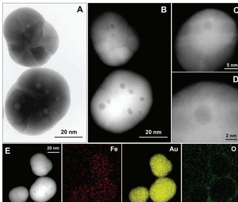
**Fig. 2** High-resolution TEM micrographs of AuFe NPs and EDX-elemental mapping. Bright-field (A) and dark-field (B) images of the same area. (C) HAADF-STEM image of another NP and the corresponding higher magnification image (D) showing continuous Au atomic columns at varying contrast. (E) STEM image and EDX elemental mapping of Fe, Au, and O in the NPs.
