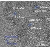
Fig. 2 TEM images (A–C) of the Si<sub>3</sub>N<sub>4</sub>/MoS<sub>2</sub> composite.
