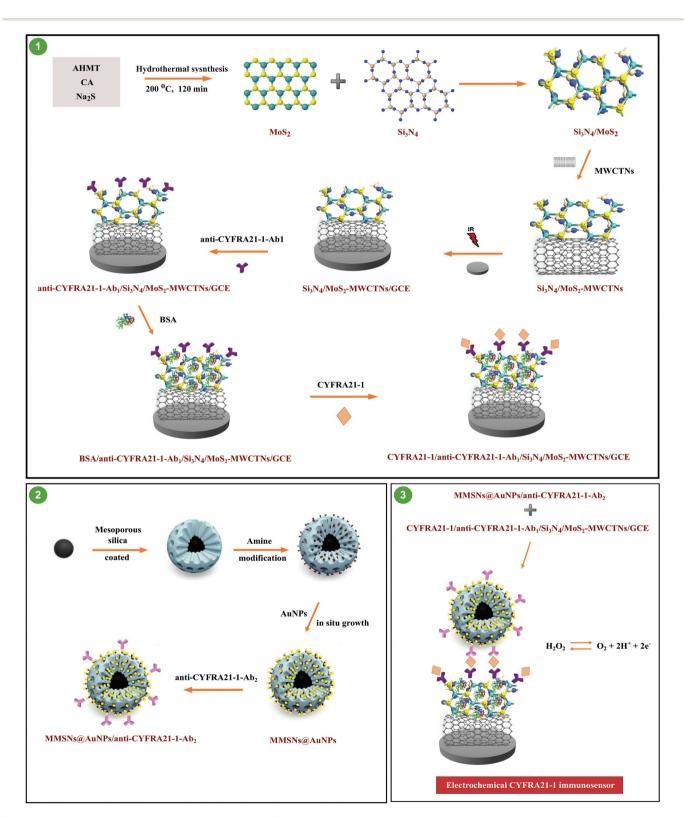
Scheme 1 Preparation procedure of the voltammetric CYFRA21-1 immunosensor.
