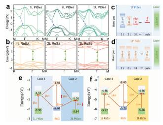
Fig. 2 The calculated band structure of 1L, 2L, 3L PtSe<sub>2</sub> (a) and 1L, 2L, 3L  $ReS_2$  (b). The energy gap at point  $\Gamma$  of  $PtSe_2$  (c) and  $ReS_2$  (d) from 1L to bulk. (e and f) Schematic illustration of the PICT process of the PtSe2-R6G system and ReS<sub>2</sub>-R6G system while the number of layers increased.
