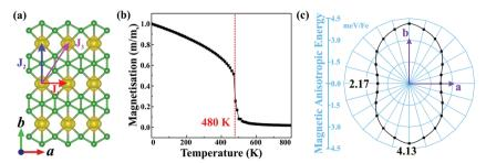
Fig. 2 (a) Spin-dependent charge density of the  $\alpha$ -FeB<sub>3</sub> monolayer, (b) average magnetic moment as a function of temperature and (c) MAE in the x-yplane with respect to the out-of-plane direction. The isovalue of the spin charge density is set to be 0.01 e  ${\rm \AA}^{-3}$ .
