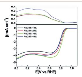
Fig. 11 RRDE voltammogram measurements of AuCNS-10%, AuCNS-20%, AuCNS-30%, and AuCNS-40%, in O2-saturated 0.1 M KOH at 2500 rpm. Reproduced with permission. 90 Copyright 2013 The Royal Society of Chemistry.
