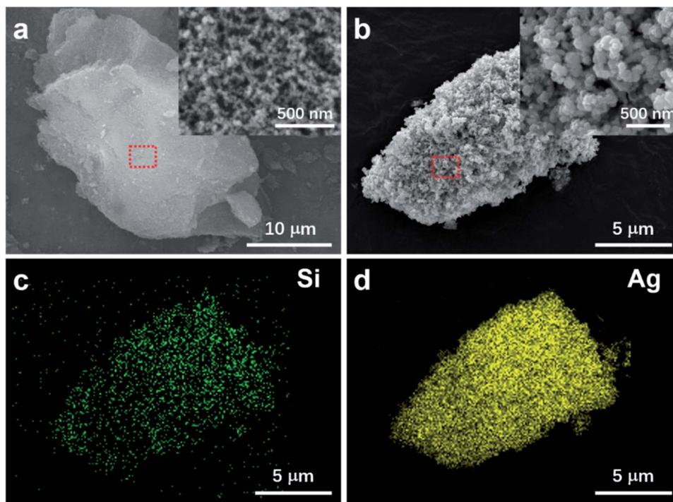
**Fig. 1** The surface morphology and elemental analysis of the AgNPs-SA powder. (a) The SEM image of the silica aerogel particle. The inset shows the corresponding magnified image. (b) The surface morphology of the synthesized AgNPs-SA. The inset shows the corresponding magnified image. (c) and (d) The elemental mappings of AgNPs-SA composite in (b) by using Si and Ag, respectively.
