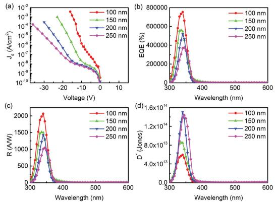
Fig. 4 (a)  $J_d$ , (b) EQE, (c) R, and (d)  $D^*$  characteristics of the fabricated UV PM-type OPDs with different active layer thicknesses. The device structure is ITO/TAPC: C<sub>60</sub>(50:1, 100 nm, 150 nm, 200 nm, 250 nm)/Al (100 nm).
