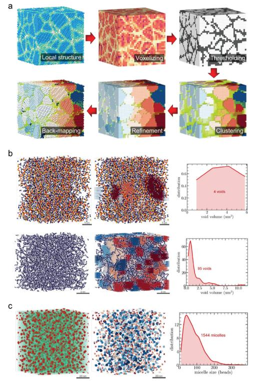
Fig. 9 An unsupervised approach for the identification and characterization of microstructures in 3-D samples of various material systems. (a) A workflow for autonomous microstructural characterization of 3-D polycrystalline solids. (b and c) Results of the ML-based microstructural analysis method on the analysis of (b) voids in porous materials and (c) micellar distribution in complex solutions (Licensed under CC-BY).  $^{176}$
