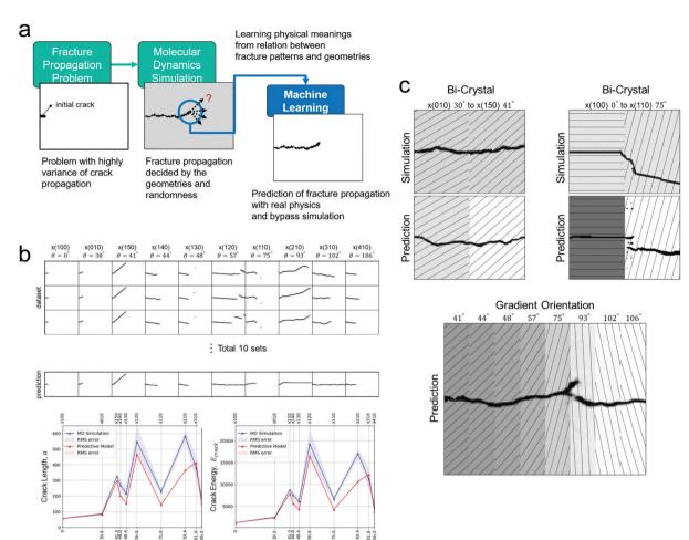
Fig. 4 Predicting dynamical fracture using a deep learning approach, dependent on microstructural details. (a) Workflow of fracture patterns prediction. (b) Comparison of crack path, length and energy release between molecular simulations and the ML approach. (c) Prediction of crack patterns in bicrystalline and gradient materials (Reproduced with permission. 114 Copyright 2020 Elsevier).
