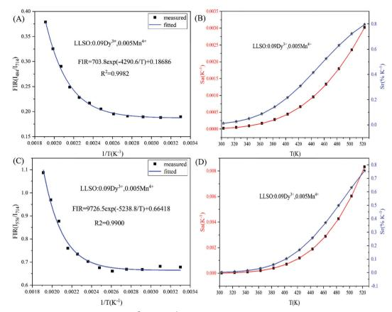
Fig. 9 FIR values,  $S_r$  and  $S_a$  values of  $La_2LiSbO_6$ :0.09Dy<sup>3+</sup>,0.005Mn<sup>4+</sup> at different temperatures.
