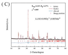
Fig. 2 Rietveld refinement patterns for X-ray diffraction patterns of (A) LLSO matrix; (B) LLSO: 0.09Tb<sup>3+</sup>, 0.005Mn<sup>4+</sup> and (C) LLSO: 0.09Dy<sup>3+</sup> 0.005Mn<sup>4+</sup>
