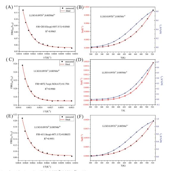
Fig. 8 FIR values,  $S_r$  and  $S_a$  values of  $La_2LiSbO_6$ :0.09Tb<sup>3+</sup>,0.005Mn<sup>4+</sup> at different temperatures.
