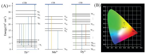
Fig. 4 (A) The light-emitting mechanism of  $La_2LiSbO_6$ :  $Tb^{3+}/Dy^{3+}$ ,  $Mn^{4+}$ : (B) CIE(x, y) coordinate diagram of LLSO:  $0.005Mn^{4+}$ ; LLSO:  $0.09Tb^{3+}$ , 0.005Mn<sup>4+</sup> and LLSO: 0.09Dy<sup>3+</sup>, 0.005Mn<sup>4+</sup>
