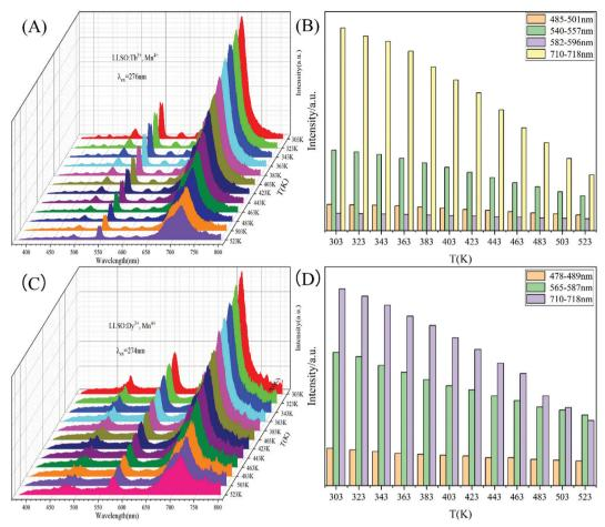
Fig. 6 The temperature-dependent PL spectra of (A)  $La_2LiSbO_6$ :  $0.09Tb^{3+}$ ,  $0.005Mn^{4+}$  and (C) LLSO:  $0.09Dy^{3+}$ ,  $0.005Mn^{4+}$ . (B), (D) The PL emission intensity of different band at various temperature.
