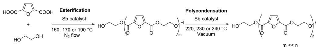
**Scheme 1** Polymerization of 2,5-furandicarboxylic acid with ethylene glycol. The first step, the esterification, affords oligomers. The second step, the polycondensation, yields poly(ethylene furanoate).
