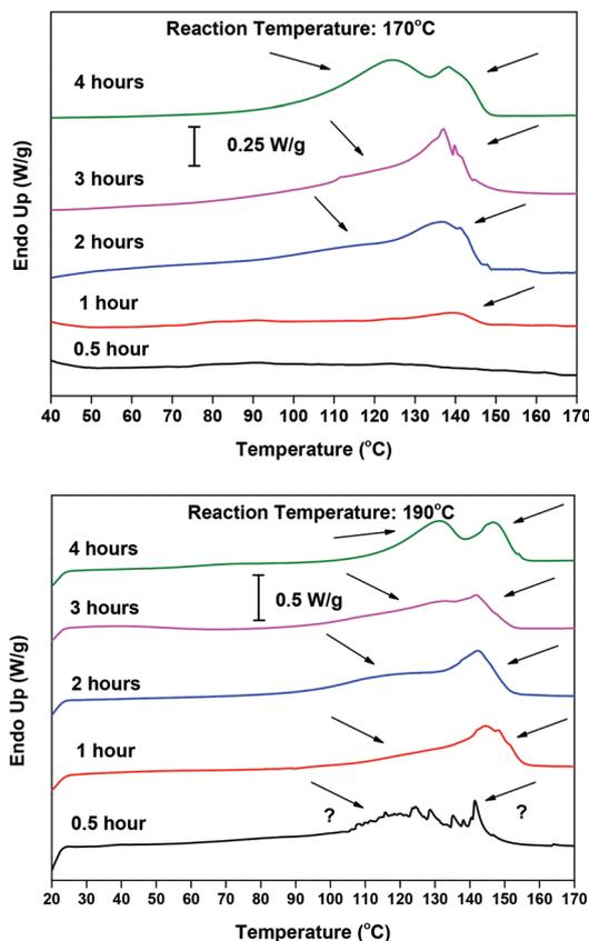
Fig. 4 DSC thermographs of the reaction samples of the esterification step, catalyzed by  $\text{Sb}_2\text{O}_3$  at  $170\text{ }^\circ\text{C}$  (up) and  $190\text{ }^\circ\text{C}$  (down), at different reaction times.
