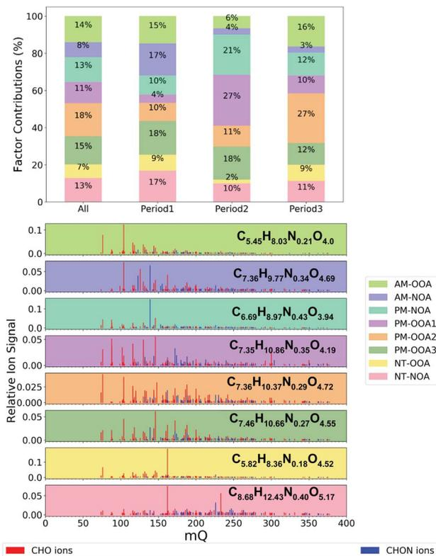
Fig. 2 Contributions of factors to total observed signal during different time periods (top) and factor mass spectra (bottom) where  $m_Q$  is the mass of the ions and the ion formulas shown are the signal weighted average ion formulas of each factor.
