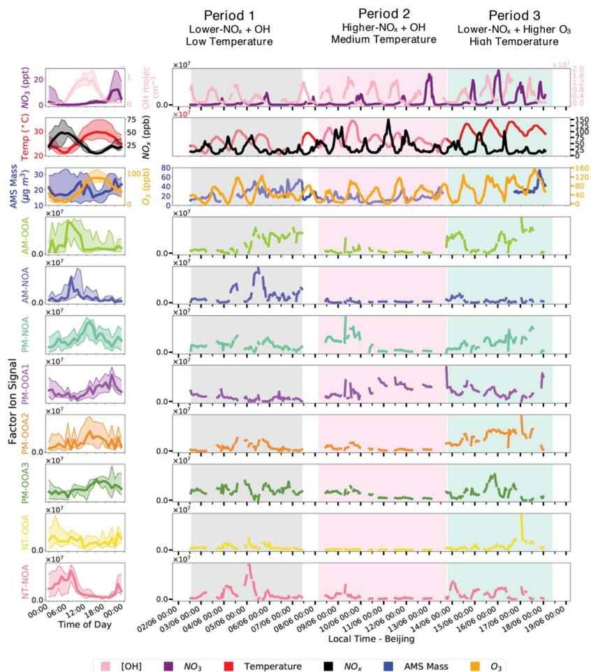
Fig. 1 Diurnal trends (left) and time series (right) of PMF factors, AMS mass, temperature, O<sub>3</sub>, NO<sub>x</sub>, NO<sub>3</sub> and OH. The PMF factors are ordered and named with a prefix according to diurnal trend that peak in the morning (AM), afternoon (PM), and night (NT).
