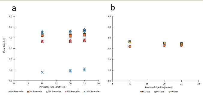
Fig. 3 a) Effect of different lengths of perforated pipe with 1.27 cm diameter holes on flow rate (left) b) flow rate vs. length of perforated pipe in 10% bentonite with different hole sizes (right).
