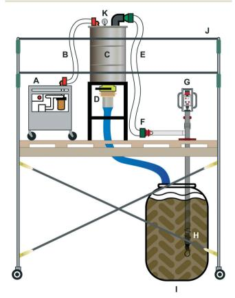
Fig. 1 Testing setup in the laboratory. A. Vacuum pump; B. vacuum hose; C. vacuum tank; D. return line to simulated pit; E. vacuum hose from excluder attachment to tank: F. cam lock connector: G. attachment motor; H. trash exclusion head; I. simulated pit latrine; J. scaffolding; K. pressure gauge.
