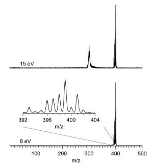
Fig. 1 Mass spectra of Ru(acac)<sub>3</sub> recorded at 8 eV and 15 eV photon energies. Only a region of the ion detector corresponding to ions coming from the molecular beam is processed for making these graphs. An enlarged section of the isotopic distribution due to the ruthenium atom is offered in the inset
