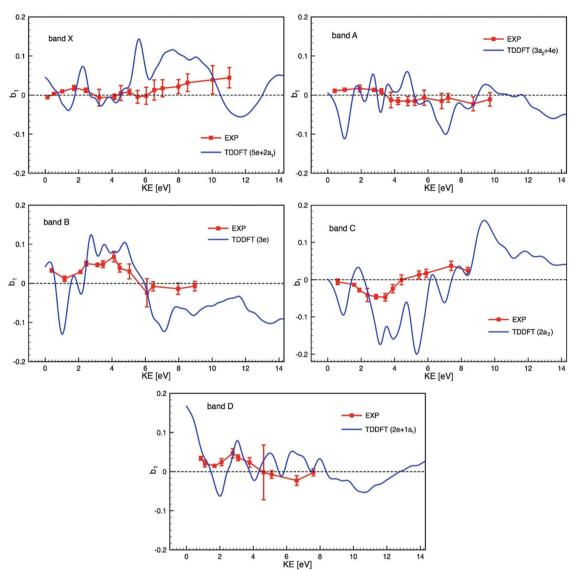
Fig. 6 Comparison of the experimental PECD data (EXP) and calculated TDDFT profiles of the dichroic parameter  $b_1$  versus electron kinetic energy (KE) for the bands X to D identified in the PES (see Fig. 3 and 4) and listed in Table 2 (the experimental data are already shown in Fig. 5). Due to the composite nature of the experimental bands (see Table 2) each calculated profile is an average over the contributing ionization channels, weighted by the corresponding calculated cross sections
