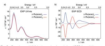
Fig. 2 Experimental UV/vis absorption (panel a) and ECD (panel b) spectra of  $\Delta$  and  $\Lambda$  enantiomers of Ru(acac)<sub>3</sub> recorded in dichloromethane (at concentrations of  $5 \times 10^{-4}$  M).
