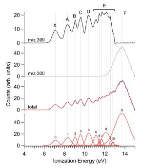
Fig. 3 PES of  $\Delta$ -Ru(acac)<sub>3</sub> recorded at a photon energy of 15 eV. The curves filtered for the parent (m/z 399, black) and fragment ions (m/z 300, grey) are given in the upper panels. The sum of the parent and fragment signals is given in the mid lower panel, together with a multi-peak Gaussian fit showing a number of visible spectroscopic features. The electronic band labels adopted for the discussion are shown in the top panel.
