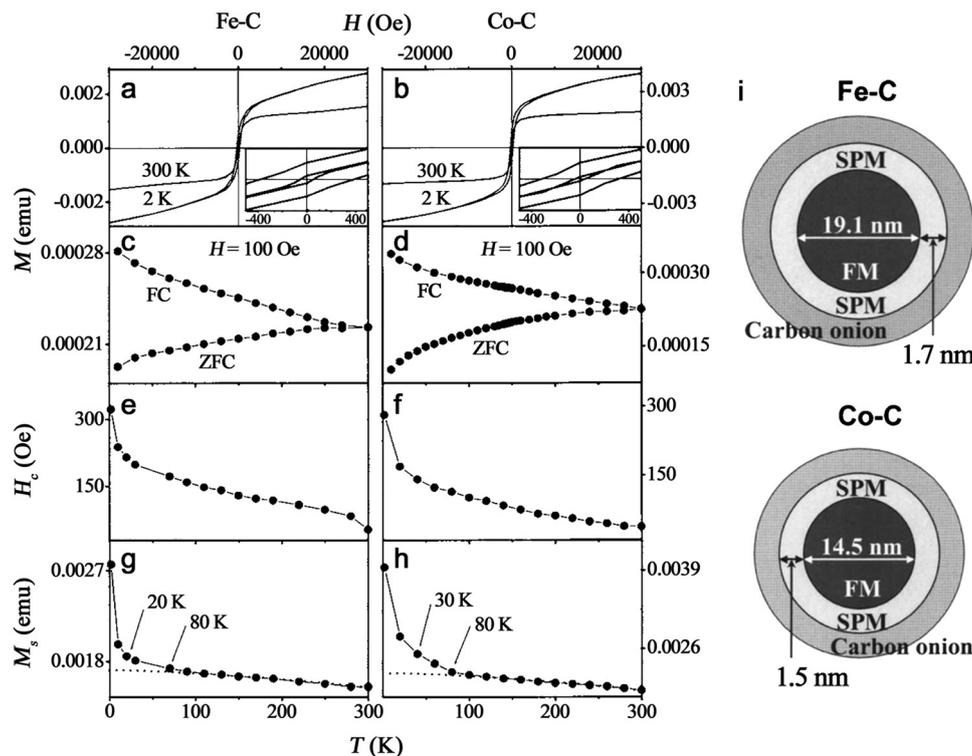
**Fig. 16** Magnetic properties of laser-generated amorphous metal carbide NPs. The hysteresis loops at 300 and 2 K of (a) Fe-C and (b) Co-C; zero-field-cooling/field-cooling (ZFC/FC) curves at  $H = 100$  Oe of (c) Fe-C and (d) Co-C; coercivity ( $H_c$ ) and saturation magnetization ( $M_s$ ) as a function of temperature of (e and g) Fe-C and (f and h) Co-C. (i) The proposed magnetic core-shell structure for amorphous Fe-C and Co-C NPs. Adapted with permission from ref. 180.
