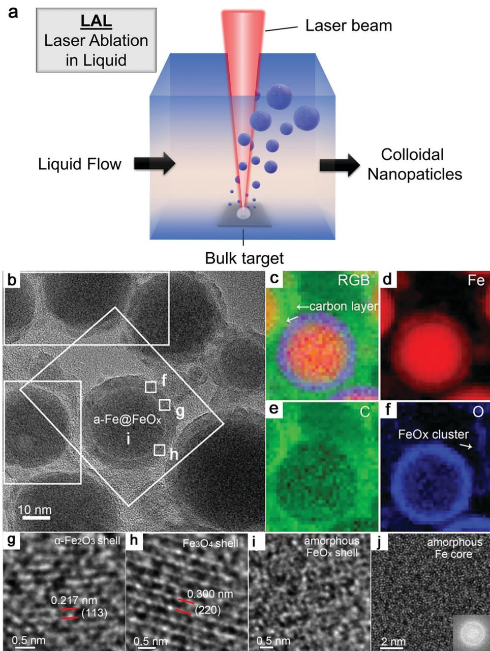
**Fig. 3** Formation of amorphous Fe oxide NPs by laser ablation in an organic solvent. (a) Schematic illustration of laser ablation in liquid. (b–f) TEM image and the corresponding EDX mapping of a Fe@FeO<sub>x</sub> core-shell NP by fs-laser ablation in acetone. (g–j) HRTEM of the selected position of the NP in (a) showing different shell structures and an amorphous core. Reproduced with permission from ref. 147.
