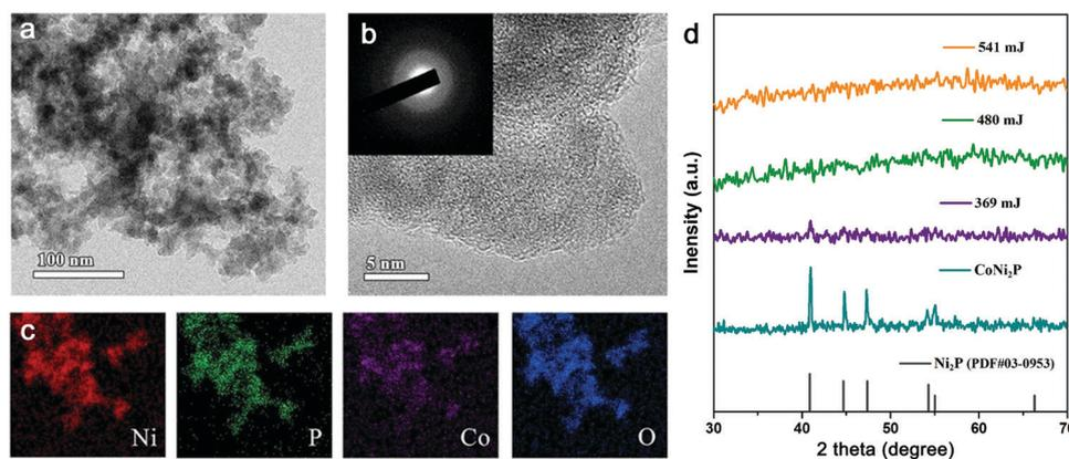
**Fig. 11** Laser fragmentation in water to synthesize amorphous multi-component metal oxide NPs. (a) TEM and (b) HRTEM images of amorphous  $\text{CoNiPO}_4$  NPs; (c) corresponding elemental mapping including Ni, P, Co and O; (d) the XRD patterns of  $\text{CoNi}_2\text{P}$  particles before fragmentation and laser-fragmented  $\text{CoNiPO}_4$  NPs under different pulsed energies: 369, 480 and 541 mJ. Reproduced with permission from ref. 203.
