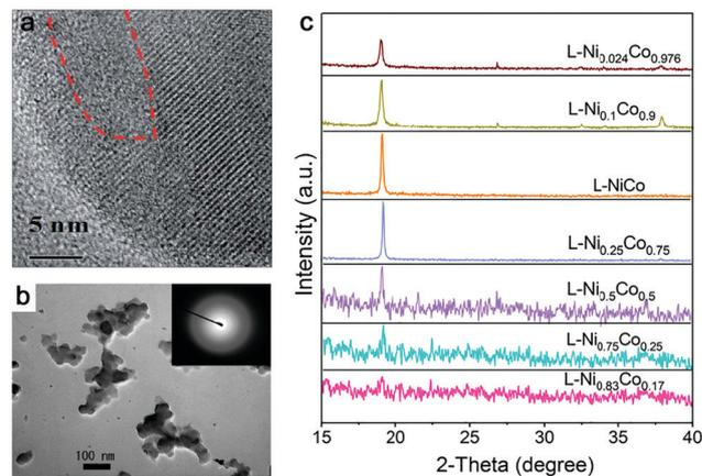
Fig. 4 Amorphous metal oxides by laser ablation in water. (a) HRTEM of FeO<sub>x</sub> NPs after laser irradiation showing some amorphous domains. Reproduced with permission from ref. 150. (b) TEM image of amorphous Pt NPs by LAL at a wavelength of 355 nm and a laser fluence of 4 J cm<sup>-2</sup>. Reproduced with permission from ref. 155. (c) XRD patterns of products with different proportions of Co and Ni by laser ablation in 1 M KOH. Reproduced with permission from ref. 159.
