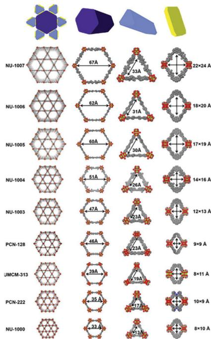
Fig. 2 Comparison of the pore size in different zirconium-based MOFs. Reprinted with permission.<sup>59</sup> Copyright 2021 Elsevier.
