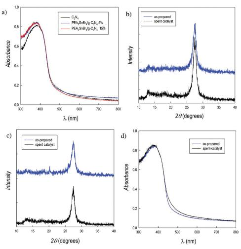
Fig. 2 (a) UV-vis spectra of pristine  $g-C_3N_4$  and  $PEA_2SnBr_4/g-C_3N_4$  composites; (b) XRD pattern of  $PEA_2SnBr_4/g-C_3N_4$  5% composite as-prepared and after the H2 photogeneration experiment (spent catalyst); (c) XRD pattern of PEA2SnBr4/g-C3N4 15% composite as-prepared and after the H2 photogeneration experiment (spent catalyst); (d) UV-vis spectra of  $PEA_2SnBr_4/g-C_3N_4$  5% composite as-prepared and after the  $H_2$  photogeneration experiment (spent catalyst).
