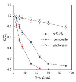
Fig. 3 Variation of MB concentration as a function of irradiation time for  $g-C_3N_4$  (blue dots) and the PEA<sub>2</sub>SnBr<sub>4</sub>/ $g-C_3N_4$  5% composite (red dots), compared to the photolysis effect (empty dots); conditions: 1 g L<sup>-1</sup> catalyst, 250 W m<sup>-2</sup> simulated solar light. RSD < 10% (n = 3).
