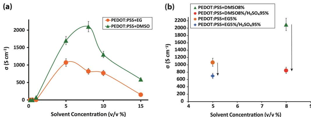
Fig. 1 (a) Conductivity values of 100 nm PEDOT:PSS thin films doped with 0.2, 0.5, 1, 5, 8, 10 and 15% v/v DMSO and EG solvents, and (b) conductivity vs. solvent concentration for the most conductive samples of PEDOT:PSS films doped with DMSO and EG solvents before and after post-treatment with sulfuric acid.
