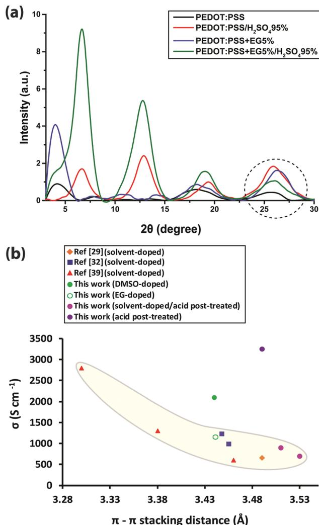
Fig. 5 (a) XRD diffractograms of pristine, EG-doped, acid-only post-treated and EG-doped/acid post-treated PEDOT:PSS films, and (b) the correlation between the PEDOT  $\pi$ - $\pi$  stacking distance and the conductivity of the PEDOT:PSS thin films.
