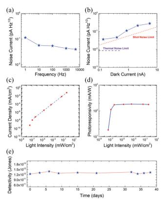
(a) Noise current measured at various frequencies in the range from 1 Hz to 5 kHz. (b) Noise current measured at different dark current levels. (c) Photocurrent density measured at varying light intensities. (d) The consistency of the photoresponsivity measured over a wide range of light intensity. (e) The detectivity of the photodetector measured over time
