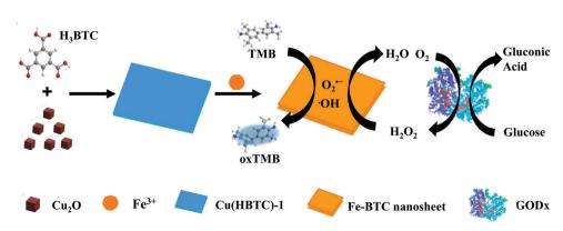
Fig. 1 Schematic of the 2D Fe-BTC preparation and its use in glucose sensing
