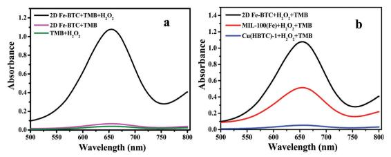
Fig. 4 (a) UV-vis absorption spectra of TMB solutions with and without 2D Fe-BTC in the absence and presence of H<sub>2</sub>O<sub>2</sub>. (b) Catalytic activities of 2D Fe-BTC, Cu(HBTC)-1, and MIL-100(Fe) under the same conditions. Reaction conditions: 0.1 mM  $H_2O_2$ , 0.1 mM TMB, and 10 mg  $L^{-1}$  catalyst for 15 min reaction at pH 3.5 (0.2 M acetate buffer) and 45 °C.
