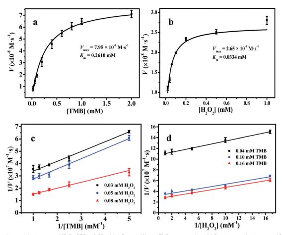
Fig. 5 (a) Steady-state kinetic assay of 2D Fe-BTC at  $0.08 \text{ mM H}_2\text{O}_2$  and different TMB concentrations. (b) Steady-state kinetic assay of 2D Fe-BTC at 0.1 mM TMB and different  $\text{H}_2\text{O}_2$  concentrations. (c) Double reciprocal plots of the 2D Fe-BTC activity at  $0.08 \text{ mM H}_2\text{O}_2$  and varied TMB concentration. (d) Double reciprocal plots of the 2D Fe-BTC activity at 0.1 mM TMB and varied  $\text{H}_2\text{O}_2$  concentration.
