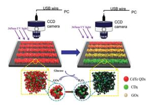
Scheme 1 Principle of the C/CdTe-GOx aerogel microsensor to detect glucose.
