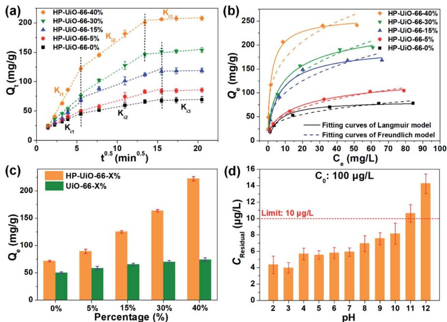
Fig. 3 (a) The As(v) adsorption kinetic curves by Weber–Morris model fitting, (b) the As(v) adsorption isotherms of HP-UiO-66-X%. (c) The uptake capacity comparisons between UiO-66-X% and HP-UiO-66-X%. (d) The effect of pH on low concentration As(v) adsorption.
